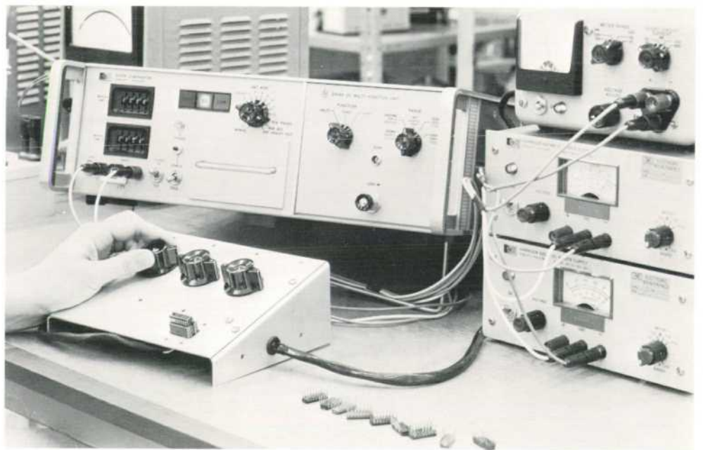
Fig. 7. Testing digital integrated circuits using a three-wafer switch to select bias levels, input levels and to scan the output of the circuits.
