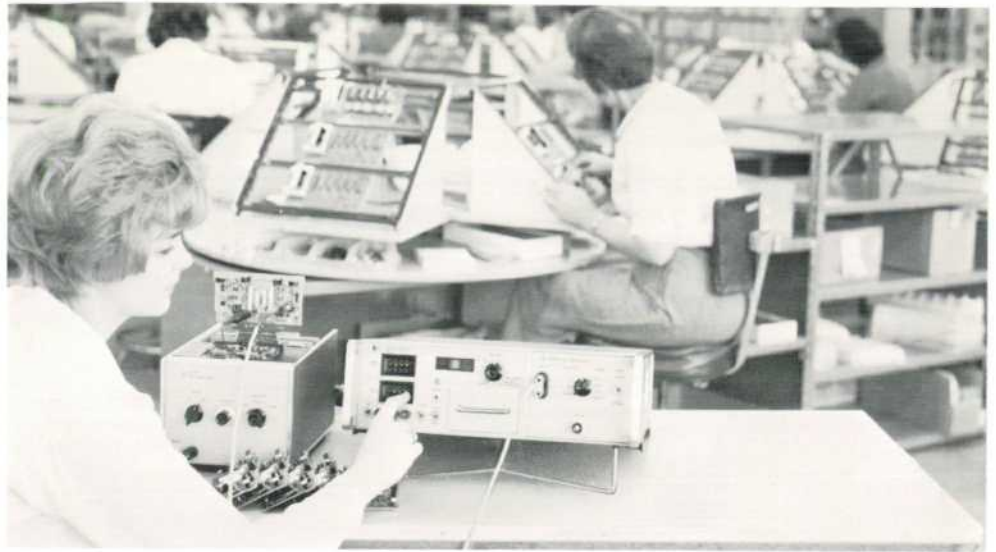
Fig. 6. Critical voltages on printed circuit boards are checked with the Comparator. Limits are set with the manual thumbwheel switches.
