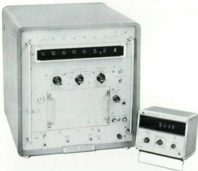
Fig. 2. HP Model 524A Vacuum-tube Counter and new HP Model 5216A Integrated-circuit Counter have comparable functions but very different sizes.
